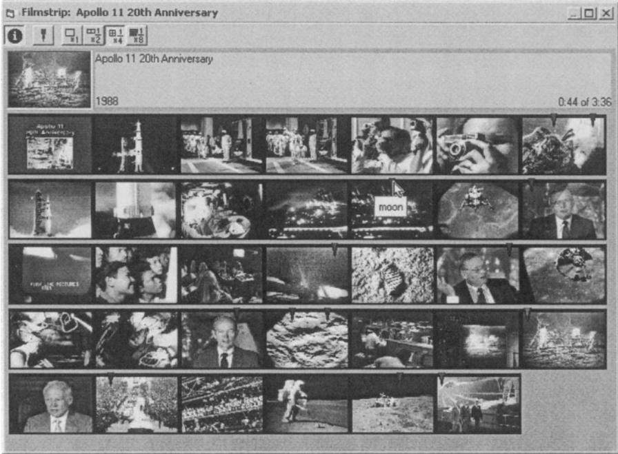
Figure 5.3 Storyboard, with overlaid match “notches” following query on “man walking on the moon.”
